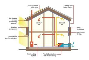
Passivhaus (or Passive House) is an advanced low energy construction standard for buildings. By using high performance insulation and effectively eliminates heat loss to create a building with very low environmental impact.
